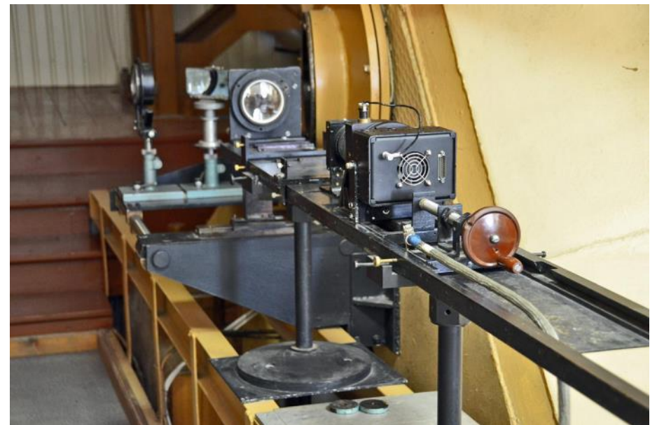
The optical bench with spectrophotometer. Photo by KY.
