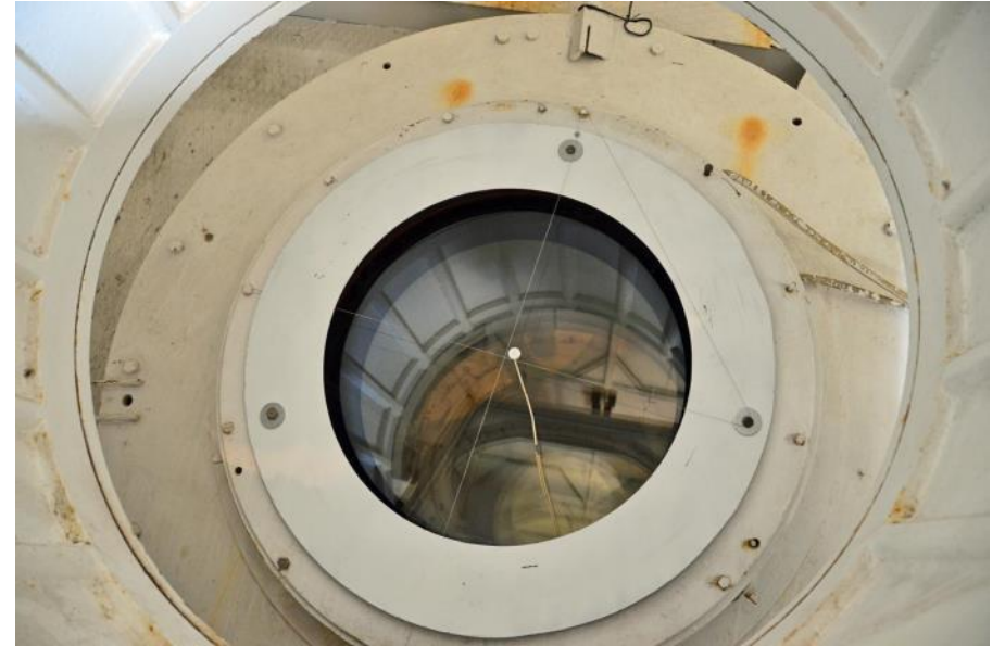
The 760 mm objective lens. Photo by KY.
