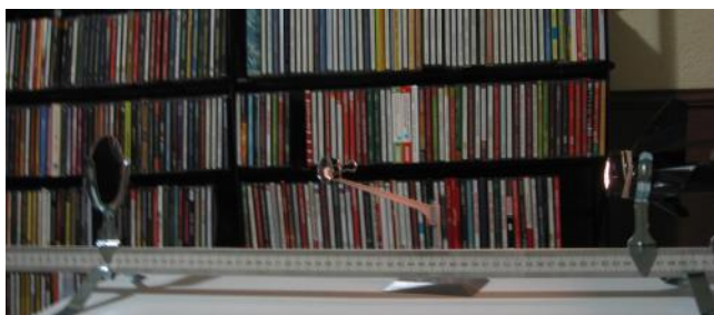
Newtonian reflector telescope: configuration of the primary (left) and secondary (middle) mirrors.
